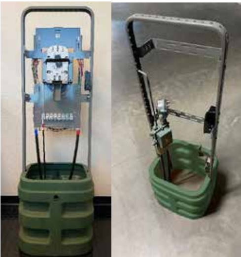
Figure 4: Fiber configuration (left) and coaxial configuration (right).
