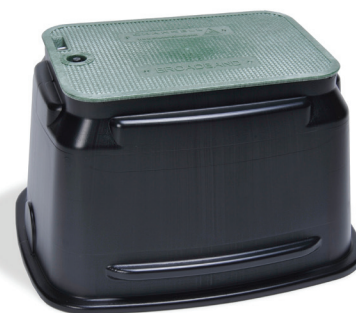
GLB1419 L-Bolt Cover Top Inside Dimensions: 10.0" Width X 15.0" Length (254.0mm X 382.0mm ) Depth: 12.0" (304.8mm) Bottom Inside Dimensions: 14.0"Width X 19.0" Length (355.6mm X 482.6mm) (Available with 6" (152.4mm) extension)
